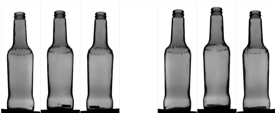
Common defects detected: stones, birds wings, seeds, dirt, fused glass, mold dope, and other opaque, aspect-related defects.
